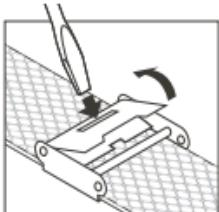
To adjust your mesh strap you need to loosen the sliding clasp. Insert a flat blade screwdriver into the rectangular slot and lever the clamp open.
