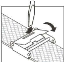
To fix the clasp in place, reinsert your flat blade screwdriver into the rectangular slot and lever it closed.
