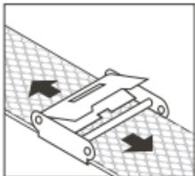
Now the clasp is free to slide along the strap to the desired position.
